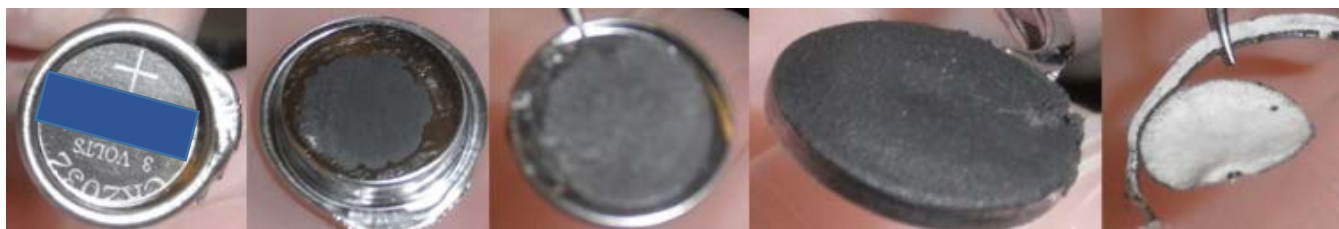
Figure 25: The CR2032 (CC02) \text{LiMnO}_2 battery and its components. Left to right: the positive side battery case, inside the positive side battery case, inside the negative side battery case, the \text{MnO}_2 electrode and the separator.
