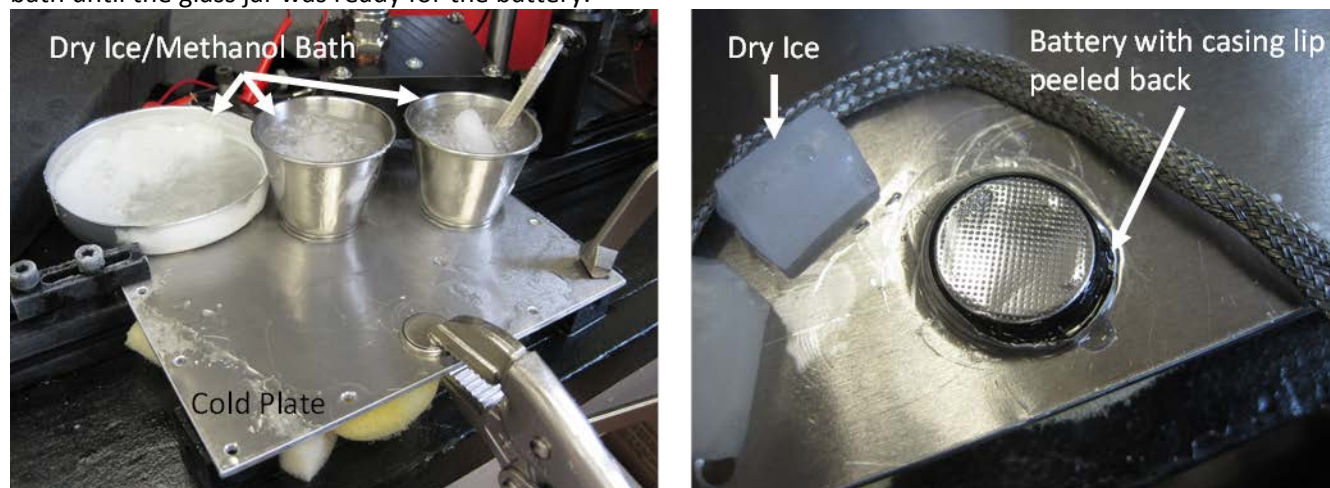
Figure 21: The left picture is the cold plate that was constructed for prying open the battery. The plate is covered with a thin layer of ethanol to maintain good thermal conduction, and the battery is clamped with a vice grip pliers. The right picture shows the battery partially opened. The procedure includes placing dry ice near the battery as the battery is opened.
