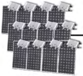
PV Modules with Microinverters
