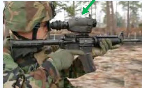
Modified MOTS TWS with embedded ATC electronics
