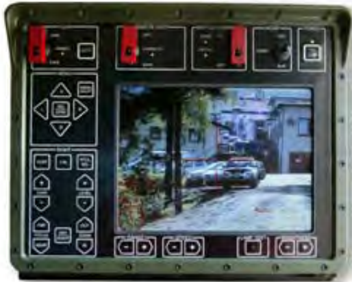
Fire Control Unit (FCU)
