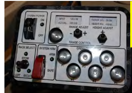
Fire Control Unit
