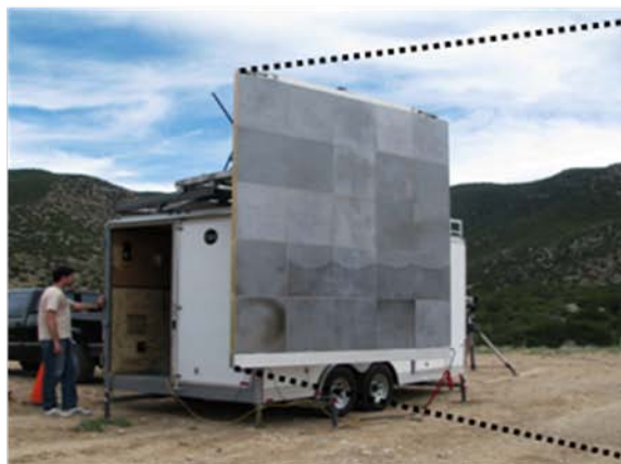
Scanning Target Board (STB) used to characterize ADS beam shape at High Energy Test Research Facility, Kirtland AFB
