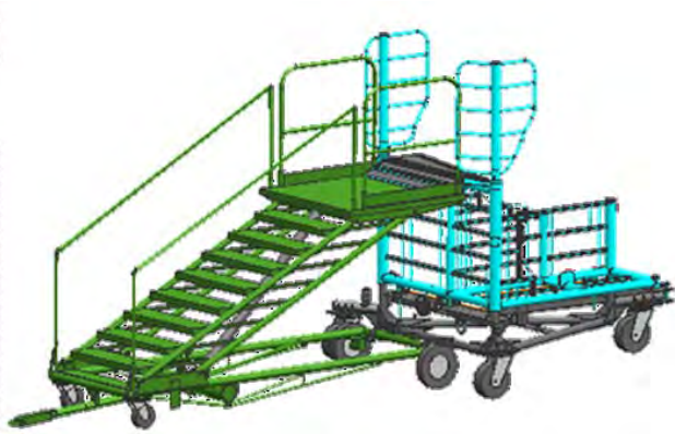
Ground Servicing Screen with B1 stand for safe cockpit exit after engine start
