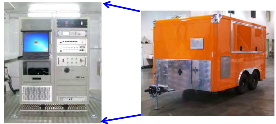
Trailer-mounted Automated System Test Set for Acceptance and Pre-Mission Testing
