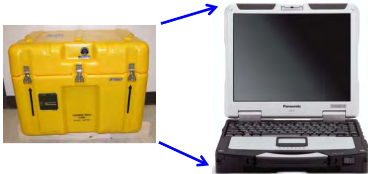
Portable Flight Line Tester for OFP load, system initialization, and diagnostics
