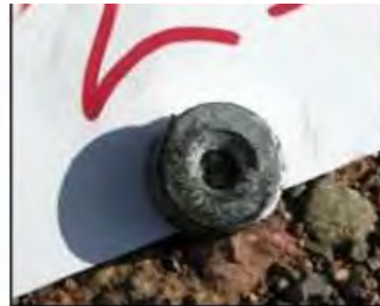
Ignition Cartridge Base at 248 feet
