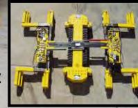
Selective Positioning Independent Deck-cargo Re-locator (SPIDR)
