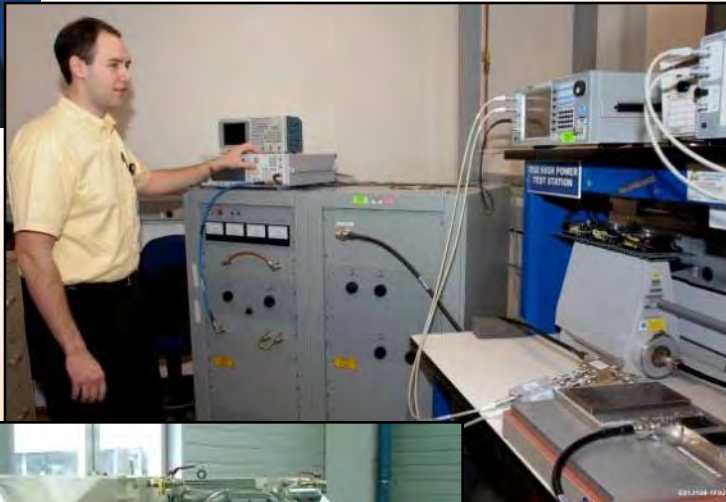
Transmit/Receive Assembly under Test
