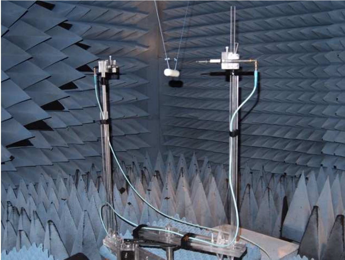
Figure 6.1: Experimental setup. The TX is on the left, the RX is on the right, and a target is visible in the top-center, hanging from the ceiling.
