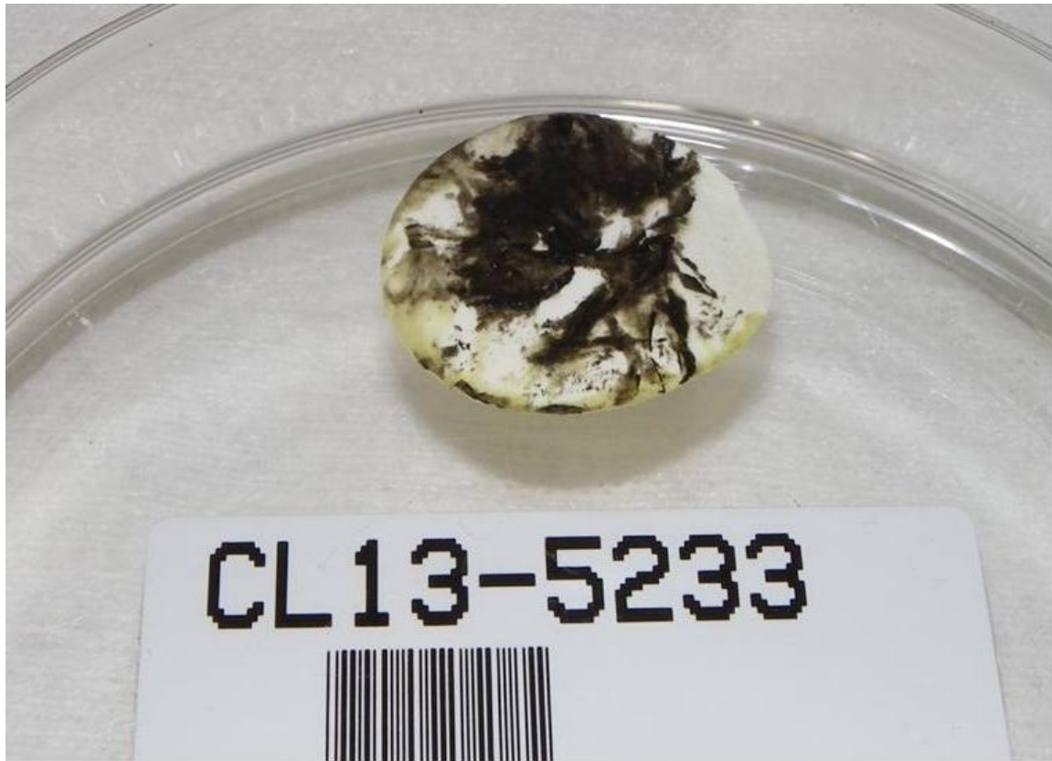
Figure 11. Scraping from HPB Media of Thickened DOT V Fluid after 11,000 Cycles
