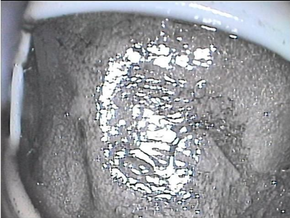
Figure 20. Filter Media after 20,000 Cycles with DOT V Brake Fluid.
