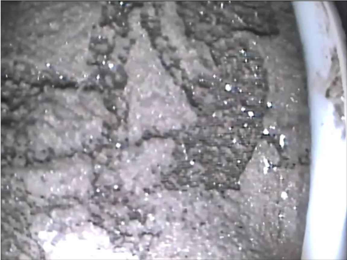
Figure 22. Heavy Deposition Noted on HPB Filter Media After 20,000 Cycles
