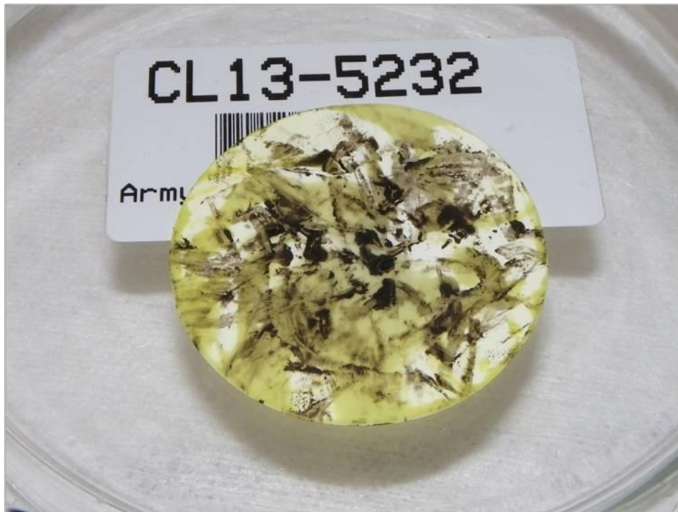
Figure 6. Scraping from HPB Media of Thickened DOT V Fluid after 7,000 Cycles
