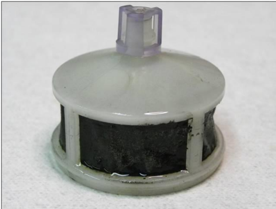
Figure 24. One of Two HPB Filter Elements with Accumulated Particulate Residue From DOT V Fluid Testing
