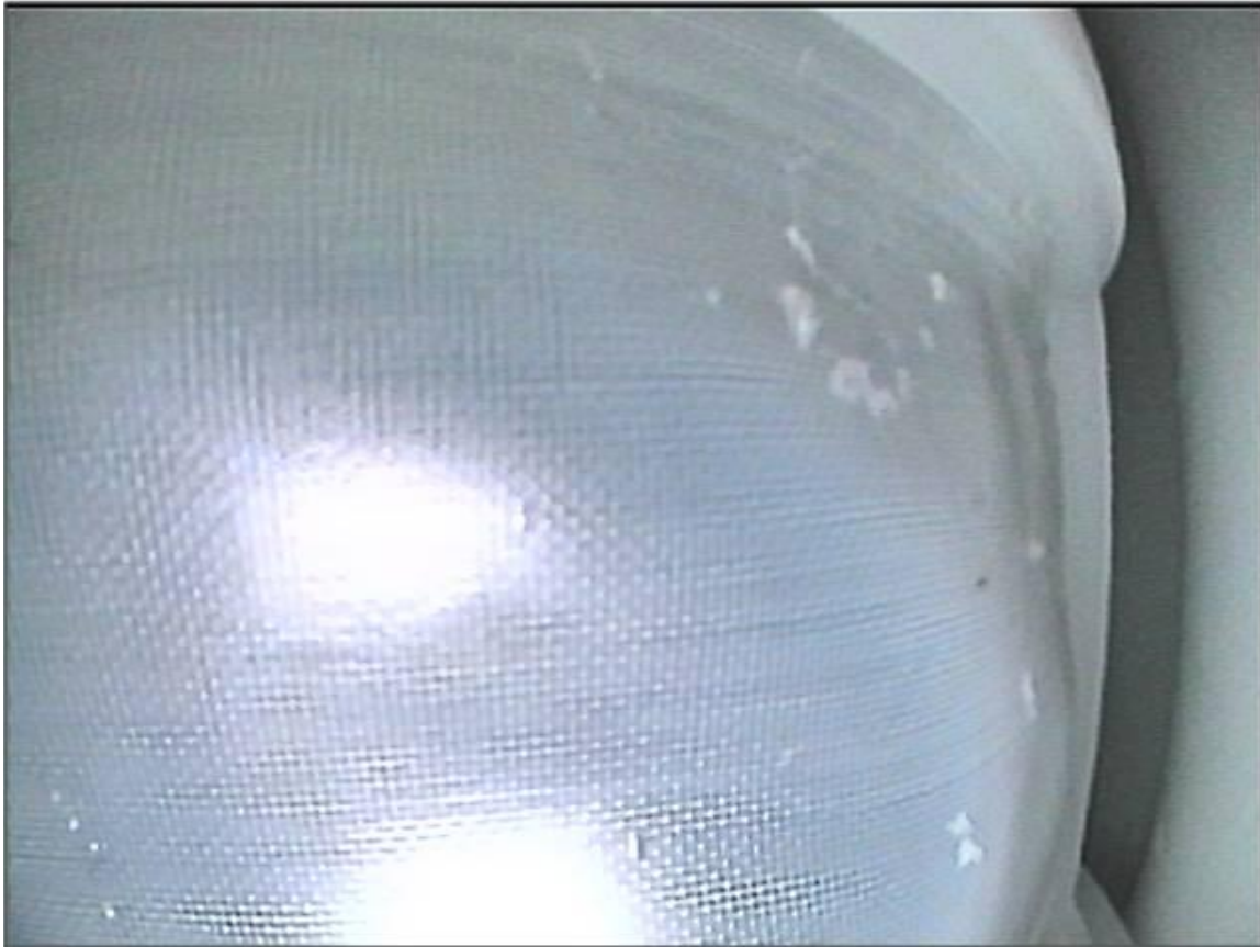
Figure 5. Clean DOT III Filter Mesh After 1500-cycles
