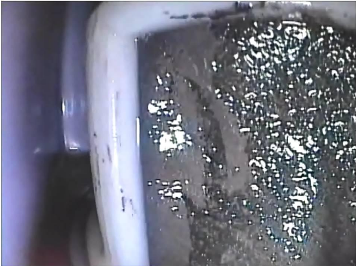
Figure 21. Image Capture From Filter Inspection Video, Revealing Deposits and Viscous Fluid Buildup
