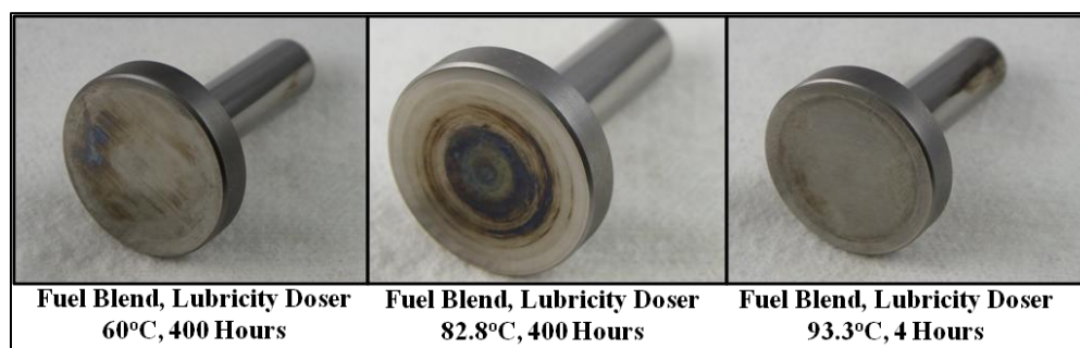
Figure 17. 50/50 Jet A/SPK Blend Component Compatibility – Upper Plunger Face
