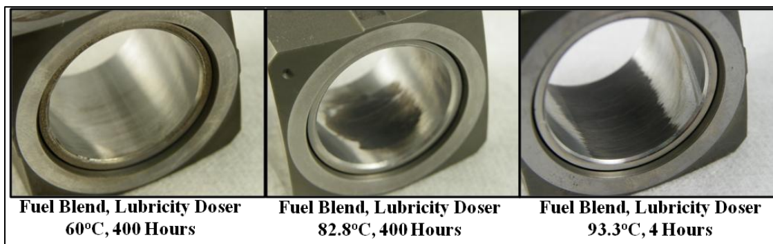
Figure 19. 50/50 Jet A/SPK Blend Component Compatibility –Ring Cam Bushing
