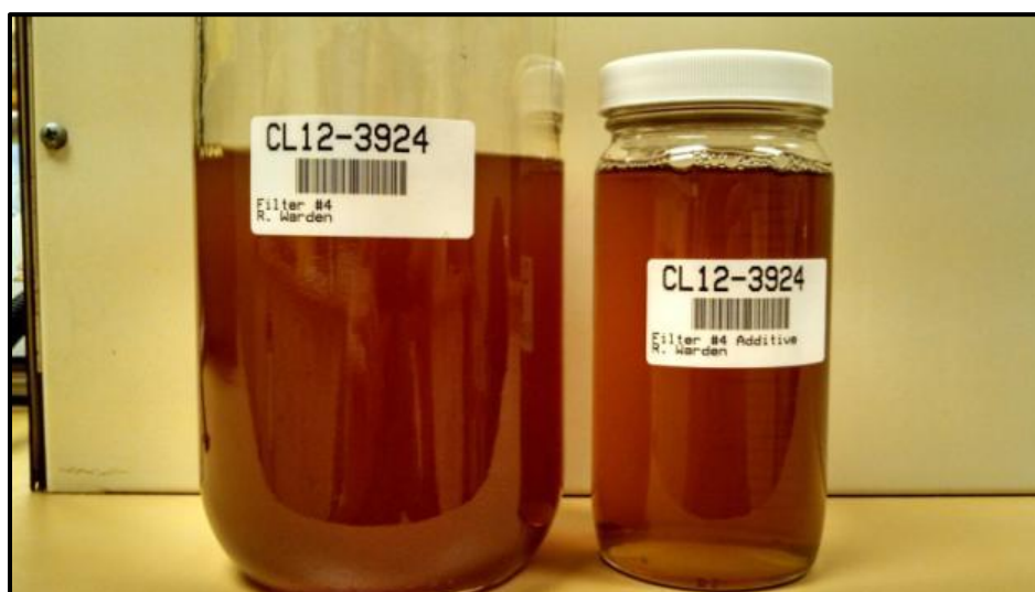
Figure 4. Storage Stability Test – End-Of-Test Fluid, Jet A in Filter No. 4
