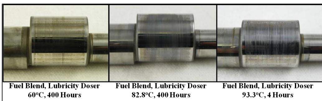
Figure 20. 50/50 Jet A/SPK Blend Component Compatibility –Cam Lobe
