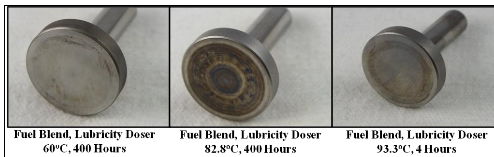
Figure 18. 50/50 Jet A/SPK Blend Component Compatibility – Lower Plunger Face
