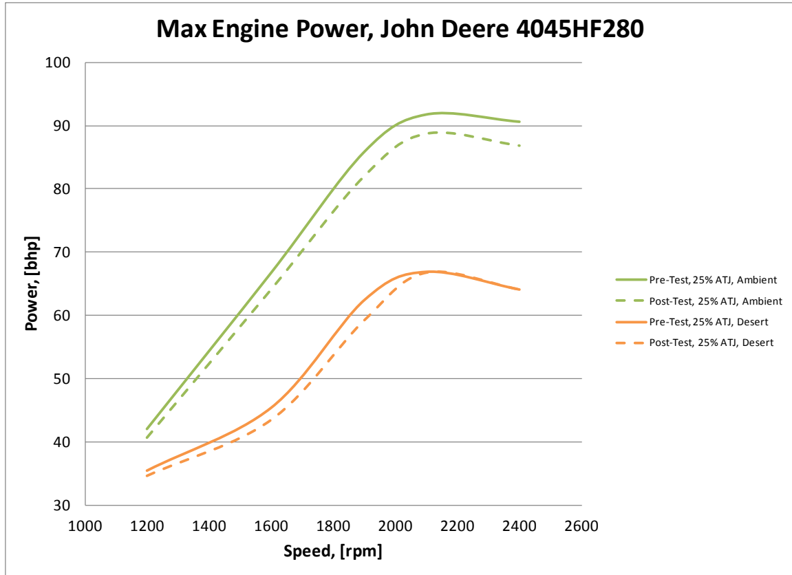
Figure 7. Full Load Engine Output, Pre-Test vs. Post-Test, 25% ATJ
