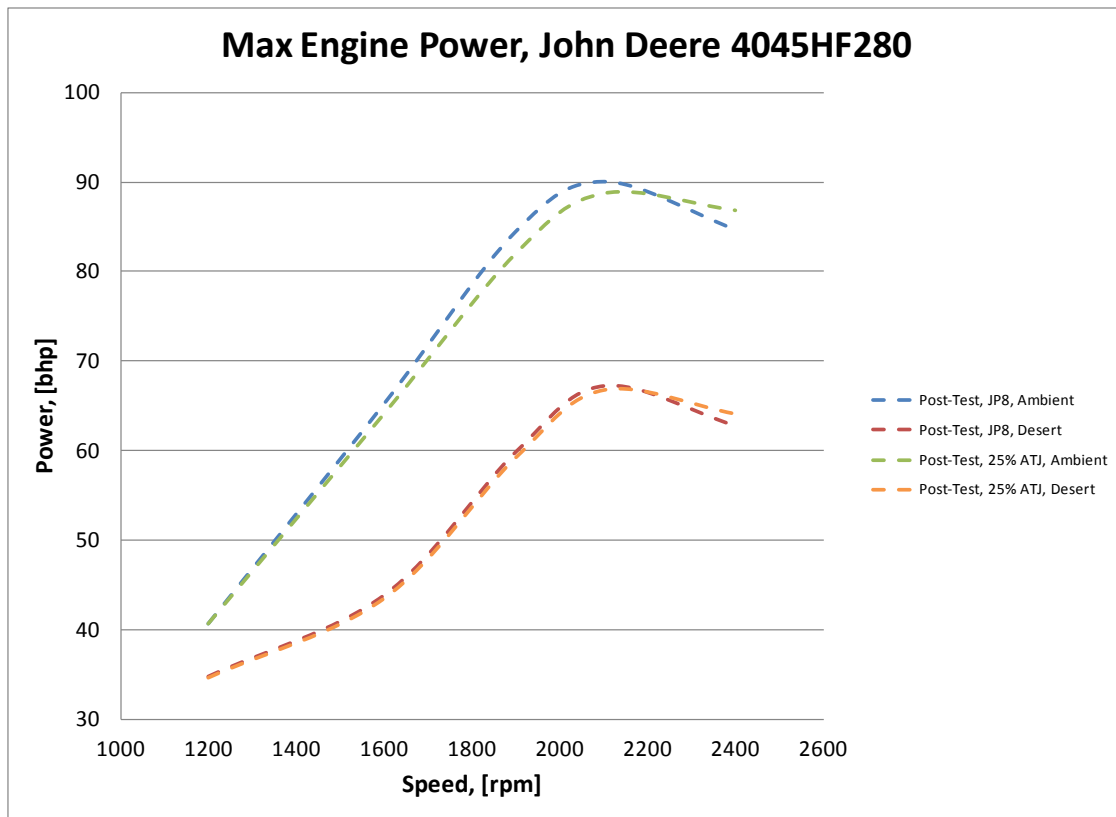
Figure 5. Full Load Engine Output, Post-Test, ATJ vs. JP8
