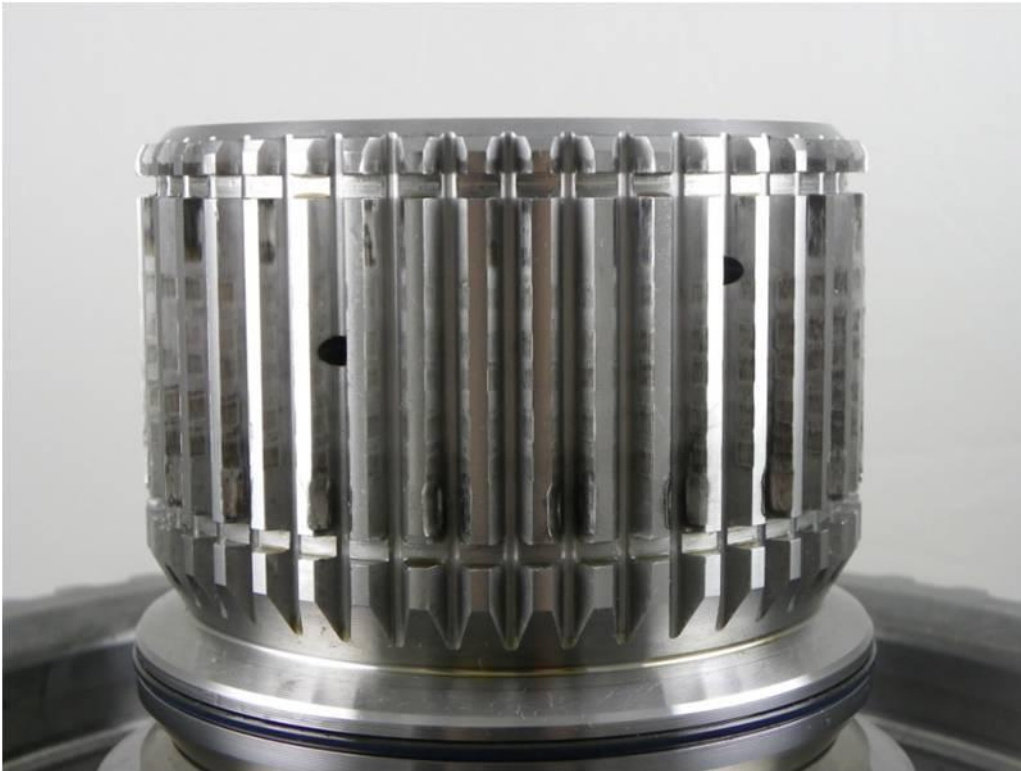
Figure 29. TEST Transmission Balance Shaft Spine Wear
