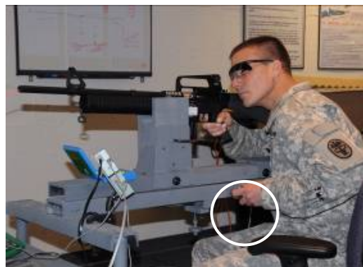
Figure 4. USAARL's purpose built gimbaled rifle mount table. The iron table's gimbaled vise rigidly secures the rifle while allowing for its aim to be adjusted both laterally and vertically. The shooter's task is to aim the rifle via set screws for vertical (elevation, left photo) and lateral (windage, right photo) adjustment and then fire the rifle. A noticeable difference in sight alignment is produced by rotating either of the set screw adjustment knobs one third of a revolution. To reduce mechanical cues, the ambidextrous set screw controls knobs are round and their action has intentional hysteresis. Cord passing through barrel on left photo is a Clear Bore Indicator (CBI) used to indicate the rifle is unloaded.
