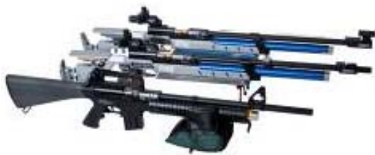
Figure 3. AiR-15 (using an Anschutz 8001 action) and Anschutz 8002 air rifles with computer scoring system. The scoring system reports each shot's score (to a 1/10 point), as well as (x, y) position (to 1/100 of a millimeter). The sights used in the study simulate M-16 (A2) iron sights, which uses the smaller long distance rear aperture of the A2 sight system.
