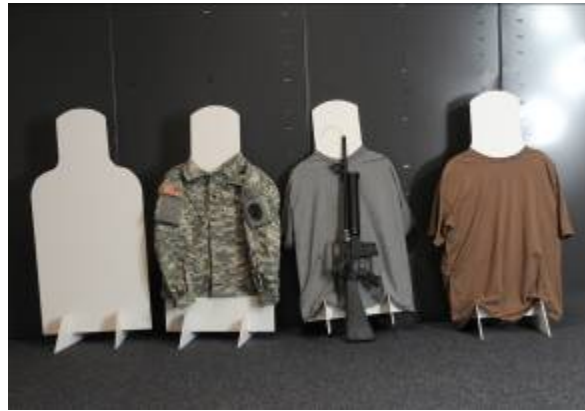
Figure 8. Examples of targets for the dark adapting task. The torso target dimensions were based on the Army's range "Target F Polyurethane 690000714589" used in rifle marksmanship training. Rifle target was an AiR-15 air rifle modeled after the M16A2 rifle, and rested across the white torso (far left) during the task.
