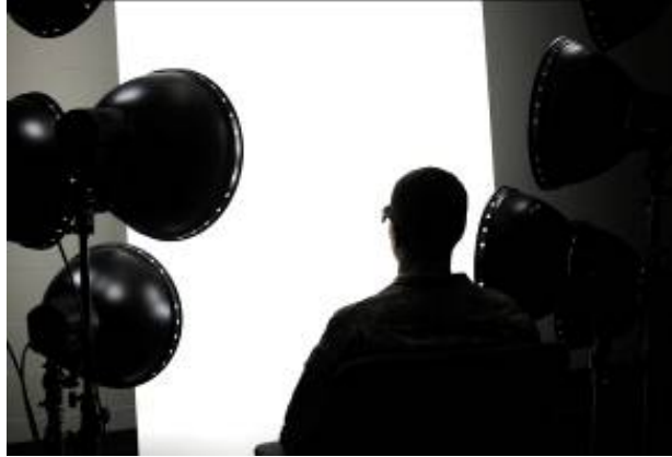
Figure 6. Pre-adapting light field approximates daylight at 1,000 \text{ cd/m}^2 . Subjects pre-adapt wearing the optical device being tested (or no device for control condition) on that run.
