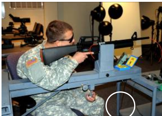
Figure 4. USAARL's purpose built gimbaled rifle mount table. The iron table's gimbaled vise rigidly secures the rifle while allowing for its aim to be adjusted both laterally and vertically. The shooter's task is to aim the rifle via set screws for vertical (elevation, left photo) and lateral (windage, right photo) adjustment and then fire the rifle. A noticeable difference in sight alignment is produced by rotating either of the set screw adjustment knobs one third of a revolution. To reduce mechanical cues, the ambidextrous set screw controls knobs are round and their action has intentional hysteresis. Cord passing through barrel on left photo is a Clear Bore Indicator (CBI) used to indicate the rifle is unloaded.
