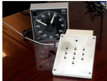
Figure 7. Purpose-built Dark Adaptometer, Control Panel, and Timer. The 10 lights on the adaptometer vary in brightness by 3.3 log units decreasing in brightness by 1/3 of a log unit from one light to the next. The control box allows any combination of the lights to be on at any given time. As subjects undergoes progressive dark adaptation, they can correctly identify the number of dimmer and dimmer lights.
