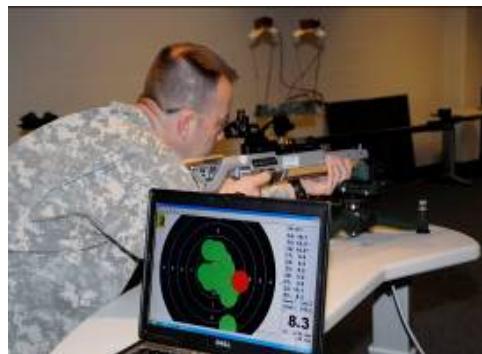
Figure 3. AiR-15 (using an Anschutz 8001 action) and Anschutz 8002 air rifles with computer scoring system. The scoring system reports each shot's score (to a 1/10 point), as well as (x, y) position (to 1/100 of a millimeter). The sights used in the study simulate M-16 (A2) iron sights, which uses the smaller long distance rear aperture of the A2 sight system.
