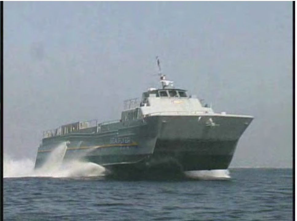
U.S. Navy Sea Flyer Large-Scale Lifting Body Demonstrator
