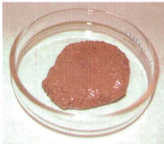
Fig. 8. Al gel produced by adding gelling polymer (1 wt%) to Al:H 2 O (1:2 wt) system.
