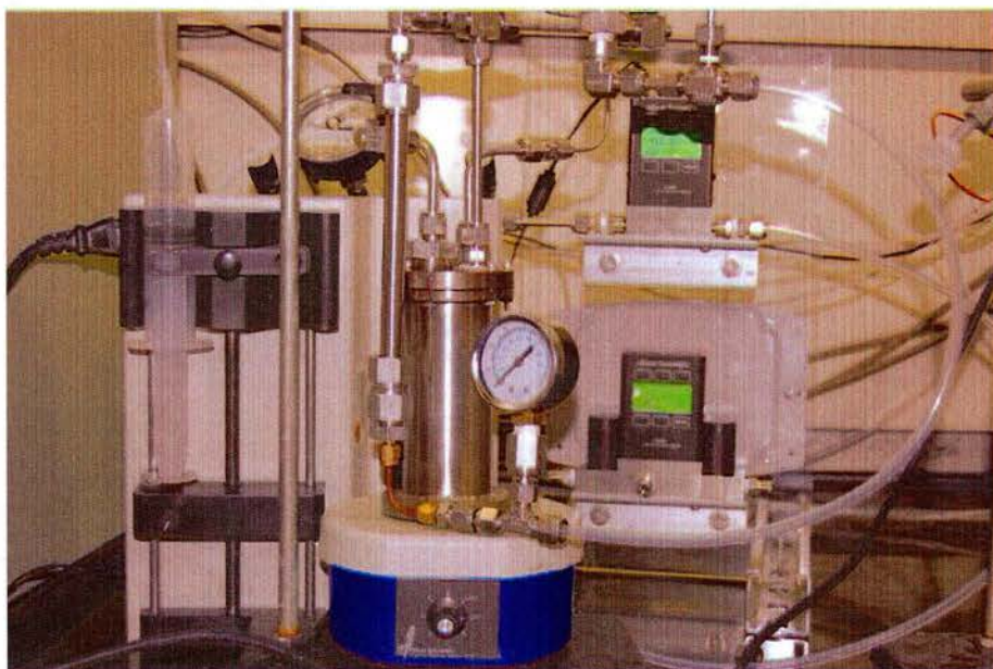
Fig. 25. Experimental setup with a stainless steel hydrolysis reactor for continuous production of hydrogen stream.
