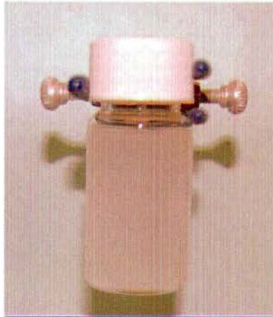
Fig. 22. NaOH-stabilized \text{NaBH}_4 dense solution ( \text{NaBH}_4:\text{H}_2\text{O}=1:2 wt) used for continuous production of hydrogen by Al- \text{NaBH}_4 hydrolysis.
