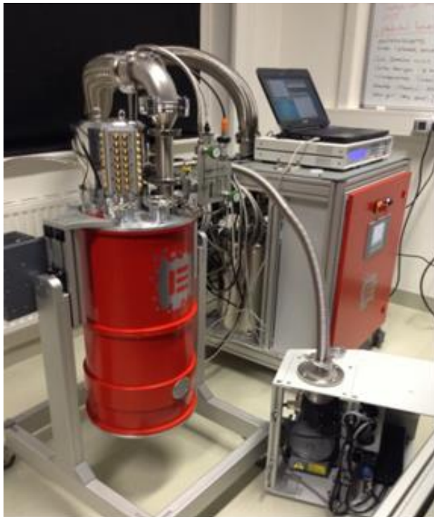
Figure 1a. Our closed cycle refrigerator. Our cooling refrigerator consists of a pulse-tube cooler mounted in a trolley with a helium compressor, buffer tank, vacuum pump station and a rack with gas handling which has the electronic control cabinet.
