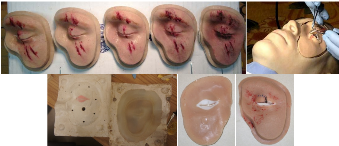
Figure 4: Top row: experiments with use of alternate silicone materials to produce correct palpation response of skin, explore cost-benefit relationship of increased realism (e.g. eye lashes, brows); original gap in face/module margin. Bottom row: modified molds showing pre-molded tarsal plate installed for overmolding process; back side of lid laceration module showing higher stiffness tarsal plate structure; front side of lid laceration module after suturing the full thickness “wound”.
