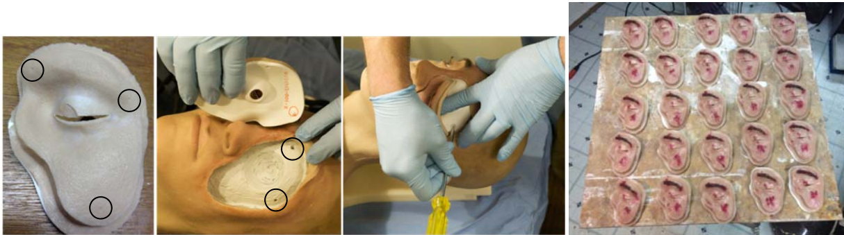
Figure 5: (left to right) Y1 module design with dimples for position calibration – instruments contact at each location to confirm position and orientation; attachment/alignment features to maintain stability of module during scenario; installation of module; 25 modules prepared for USUHS user testing.
