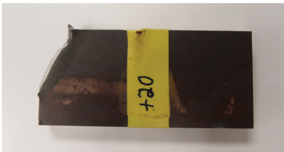
Figure 4.26: Drop Tower Specimen – Ductile Failure – View 2
