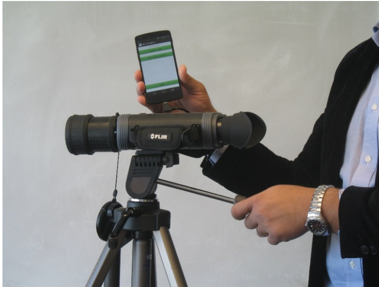
Figure 3. The integrated imaging system, without the Android device mounted on the camera. The camera is shown with a 100-mm lens. The camera is on a tripod, although it can also be used in a handheld mode. The Android device displays the user interface for the custom Camera Controller application.
