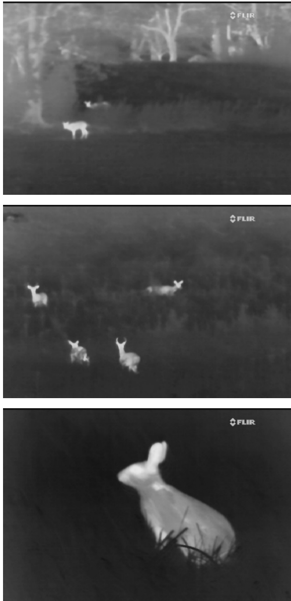
Figure 1. Example images from the FLIR BHM-6XR+ infrared camera. These were captured soon after sunset with a 100-mm lens. Each image is 720 x 480 pixels in size, and is in JPEG format.
