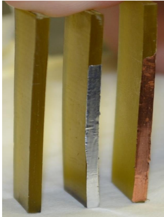
Fig. 1 JA2 samples (left to right) with no foil, Al foil, and Cu foil
