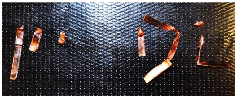
Fig. 8 Copper remains at 8.68 MPa; left is 2-mil Cu, right is 3-mil Cu
