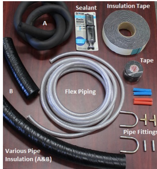
Figure 33. Parts required for cooling system construction
