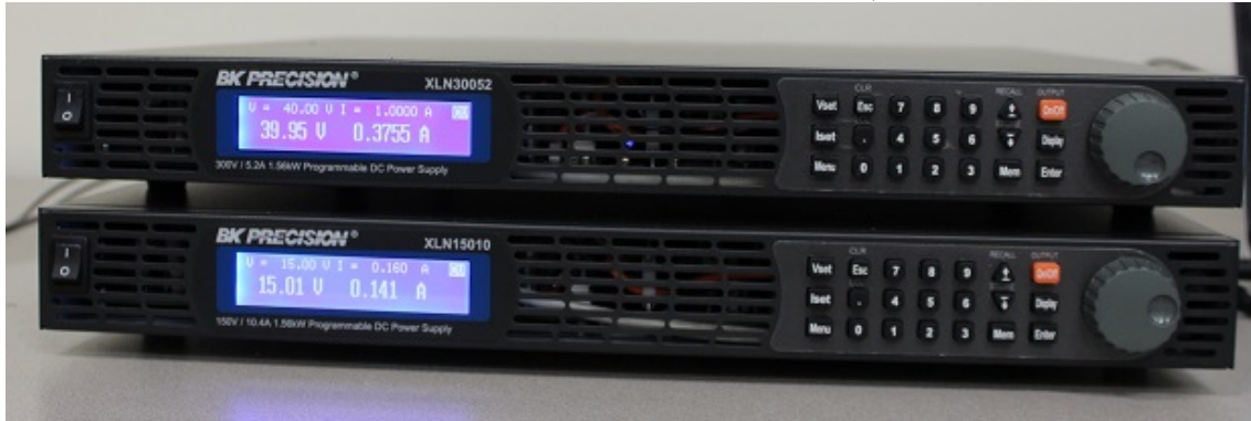
Figure C.C.1. BK Precision High Power Programmable DC Power Supply (Model XLN30052 and XLN15010 shown)
