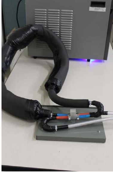
Figure 35. Fully assembled cooling system
