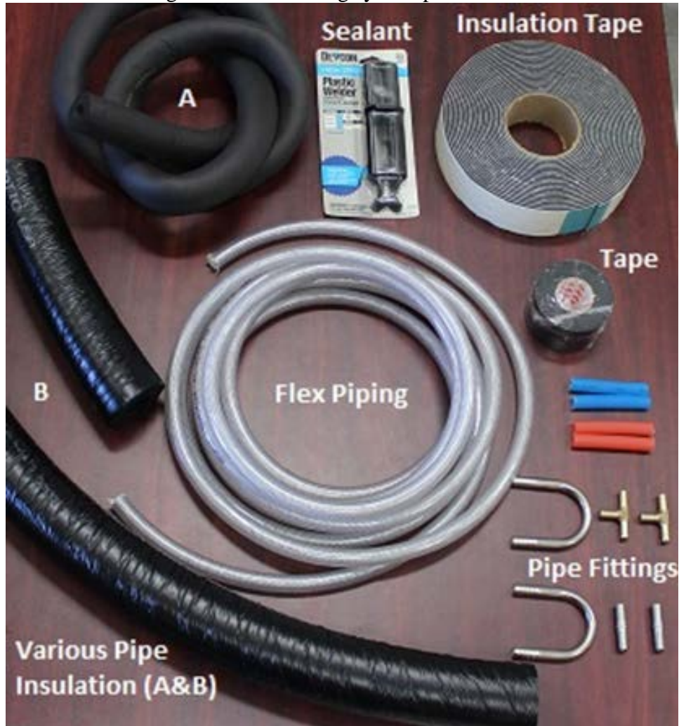
Figure B.A.1. Cooling system parts needed
