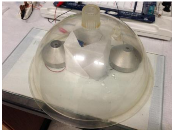
Figure 79. NTSDM capacitor test assembly with humidity control cover.
