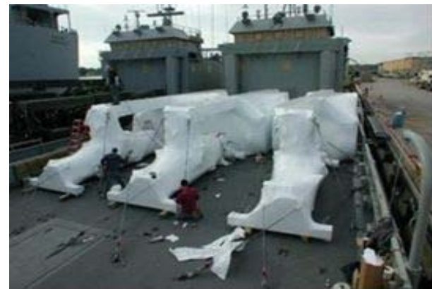
Effective shrinkwrap allowing safe deck top shipping
