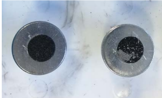
Figure 15. SEM Samples Stubs prepared for Analysis. “Wet” Preparation (left) and “Dry” Preparation (right) are Both Shown in this Image
