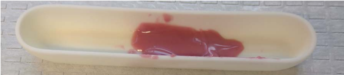
Figure 11. Precursor Slurry in Alumina Boat for Heating
