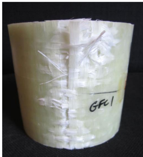
Figure 46. Glass Fiber Composite #1 Failure Location.
