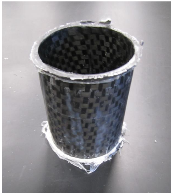
Figure 27. Rough Carbon Fiber Composite Cylinder after Removal from Mold.
