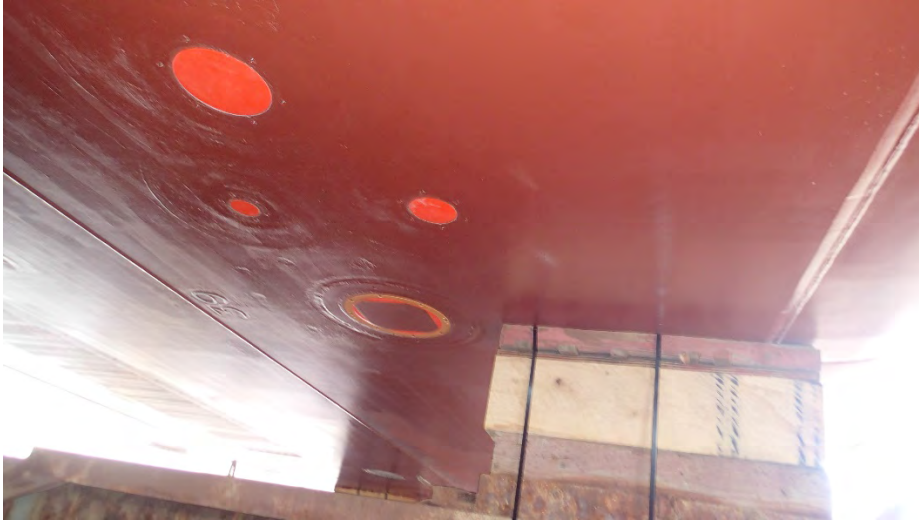
Figure 1EK80 Single Beam Transducers This is prior to the yard adding a light coat of AF.
