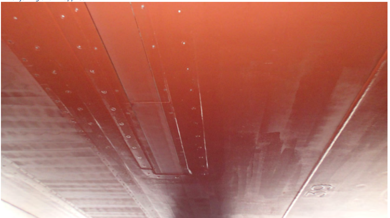
Figure 2EM712 With fairing and AF applied.
