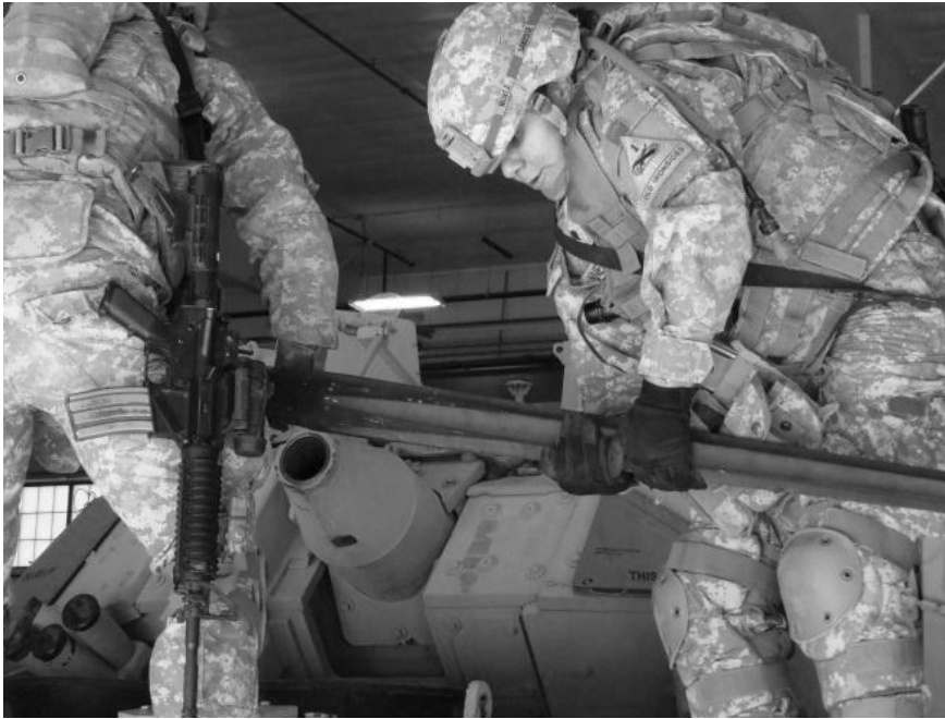
Figure 1.5. Image of Soldier Installing the Barrel of the 25mm Gun on a BFV (Task 5)
