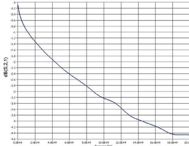
Figure 468: Measured loss of the RF cable after the LNA (probe arm C2 plus 36 inch cable).
