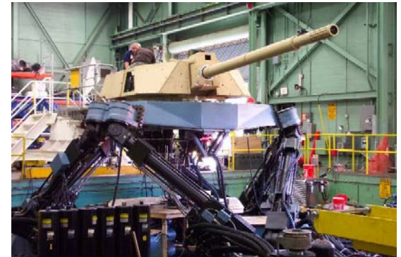
Firing Platform on TMBS at TARDEC
