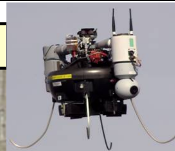
Class I Block 0 with Gimbaled sensor
