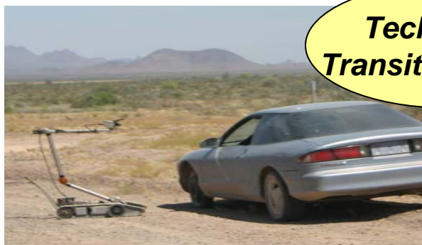
Integrated Nomadics Fido XT on iRobot Packbot EOD variant
