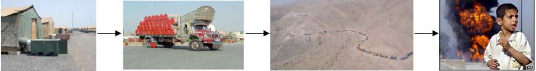
One inefficient 5-ton a/c uses ~1 gal/h of genset fuel. Truck's 68-barrel cargo can cool 120 uninsulated tents for 24 h. This 3-mile convoy invites attack. (Photos aren't all in the same place.)
