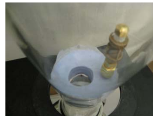
Standard Grade RP-1 after extraction with 10:1 IPA water in extraction apparatus
