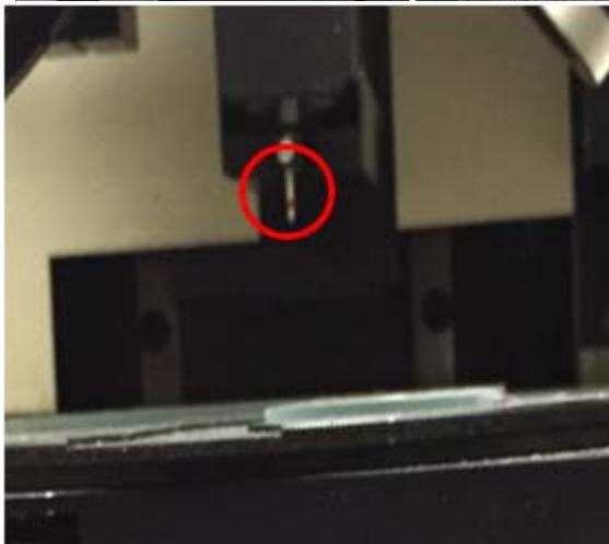
Figure 3. The stylus that moves across the sample is circled in the picture. The Dektak 3 is a stylus based surface profiler. This means that the stylus is in physical contact with the sample. The radius of the standard stylus in our setup is 12.5 microns (as indicated by the red band around the stylus). This size meets most of the samples measurement requirements. However reducing the tip size necessitate the changing of the stylus force to a lower value.
