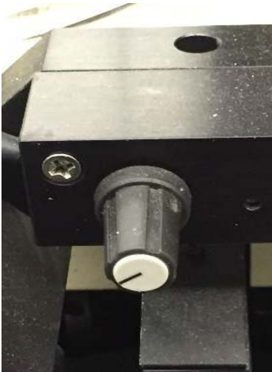
Figure 7. Sample illumination is controlled by the illumination control knob. Turning it clockwise will increase the intensity of the light. Turning it completely counterclockwise will turn off the light.
