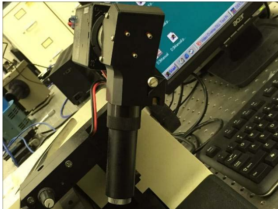
Figure 1. The 90X solid state video camera with a variable intensity illuminator in the setup can be used to view the sample placed on the sample stage.
