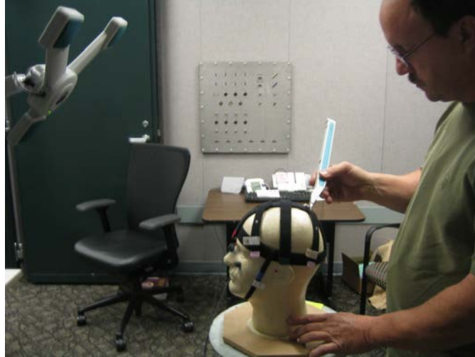
Fig. 3 Digitization of electrode positions with the zebros ELPOS ultrasonic system
