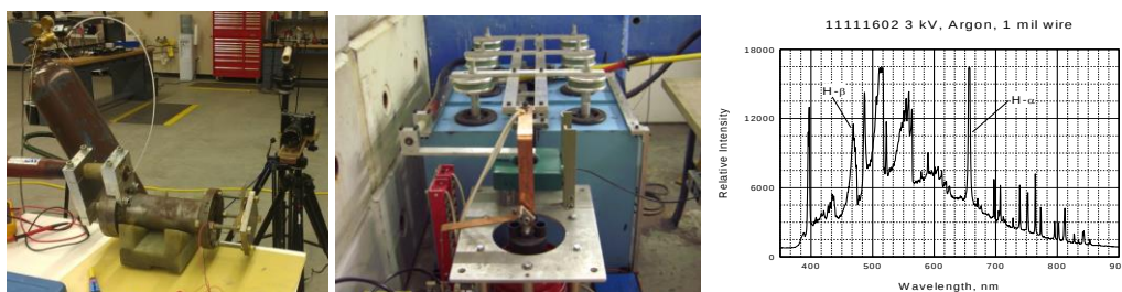
Figure 1: Capillary discharge (left), power supply for the capillary discharge (middle), and a spectrum used to establish plasma temperature and electron density (right).
