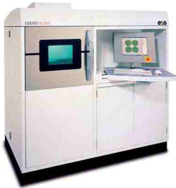
FIGURE 3.24: EOS M280 DMLS platform was used to manufacture the micrometer supersonic gas jet.
