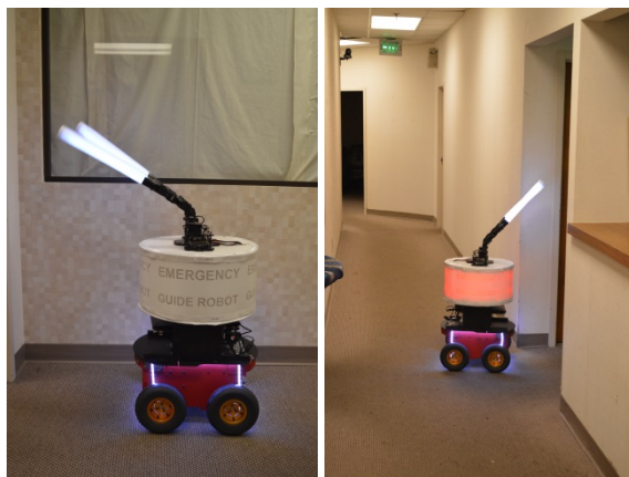
Figure 32: Robot during non-emergency round pointing to meeting room door (left) and robot during emergency round pointing to back exit (right). Note that the sign is lit in the right picture. A standard emergency exit sign is visible behind the robot in the emergency round.
