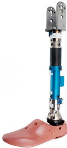
Figure 1. MIL-LX, which uses the midsize-male Hybrid-III foot (Humanetics Innovative Solutions).
