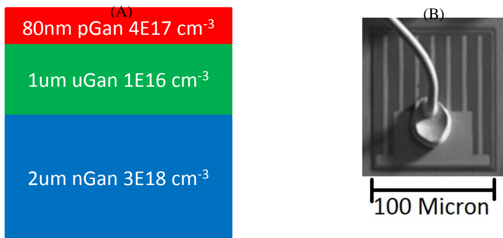
Fig. 3 A) Doping profile diagram and B) SEM image of GaN device evaluated composed of p-type (80 nm thick), undoped region (1 um thick), and n-type region (2 um thick)
