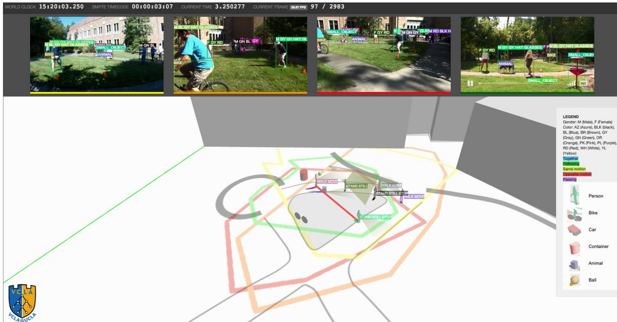
Figure 56. The garden scene. 3D space and time parsing the scene and events by integrating images from multiple cameras.
