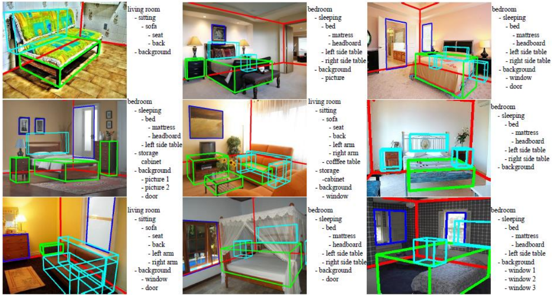
Figure 36. Parsing results include cubic objects (green cuboids are detected by bottom-up step, and cyan cuboids are detected by top-down prediction), planar objects (blue rectangles), background layout (red box). The parse tree is shown to the right of each image.
