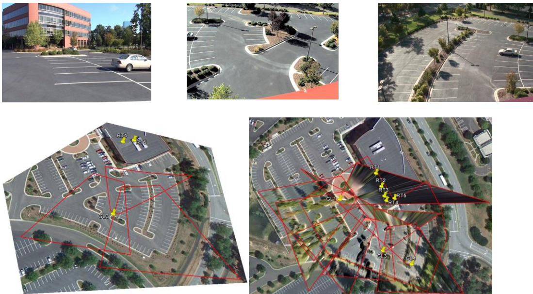
Figure 19. Geo-registration of three camera views (top) at the parking lot scene. (bottom-left) The three pins show the camera positions and the red polygons are the ground seen by the three cameras. (bottom-right) More views are registered to the map.
