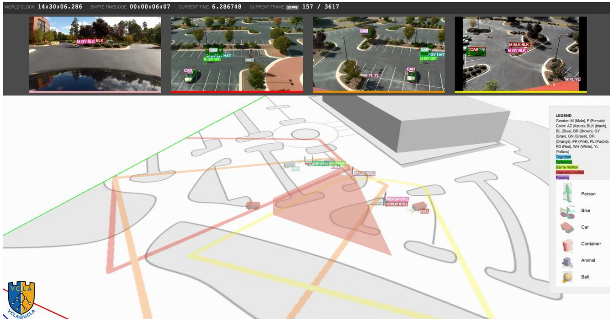
Figure 55. The parking lot scene with a moving camera (the upper left) mounted on a vehicle. 3D space and time parsing the scene and events by integrating images from multiple cameras.
