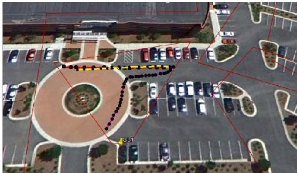
Figure 25. Tracked object trajectories transformed from the 2D camera view to the 3D world coordinate frame.
