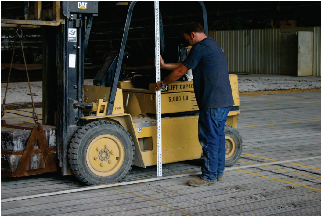
Figure 39. Loaded deflection procedure used to determine \delta_{s-2} .
