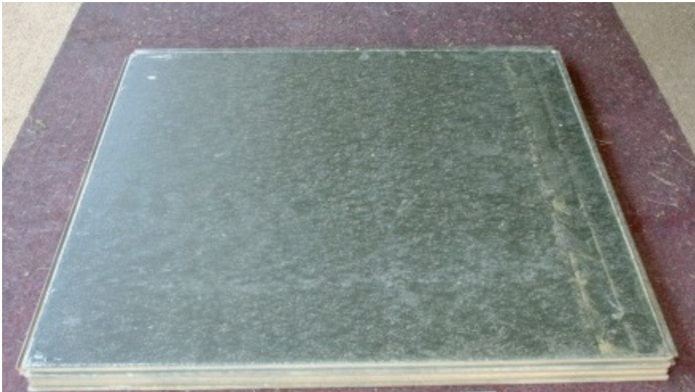
Figure 6. M19 mat panel.
