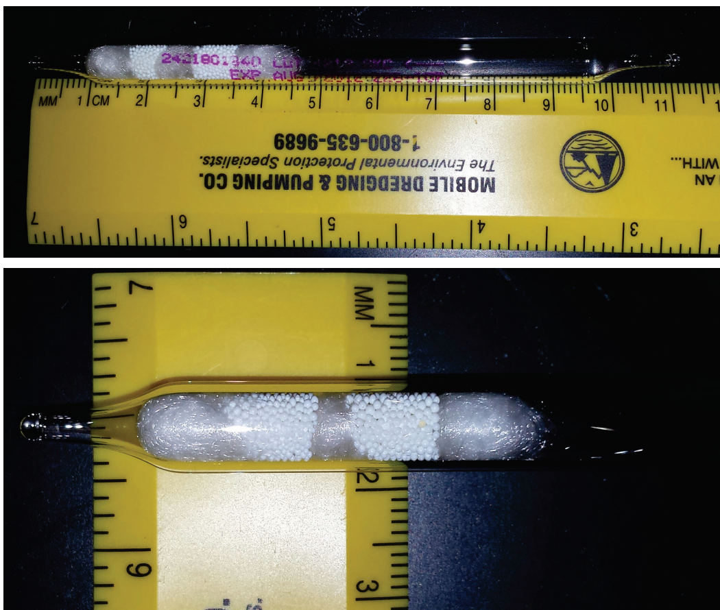
Figure 8. Sorbent tubes used as after-column traps in column experiment.
