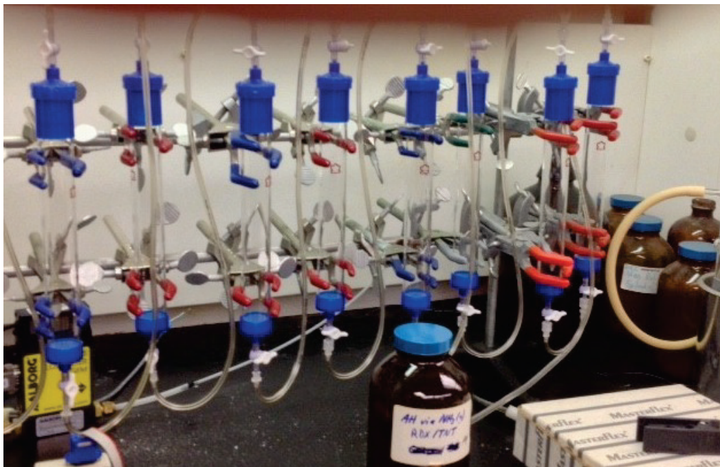
Figure 7. Set up for column study. Columns were set up to flow in series.
