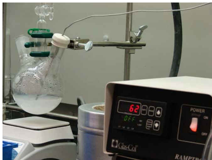
Fig. 5.2. Synthesis of chitosan/ \text{LaF}_3 : \text{Ce}^{3+} NCs: The solution undergoes cooling down to room temperature after the synthesis period.
