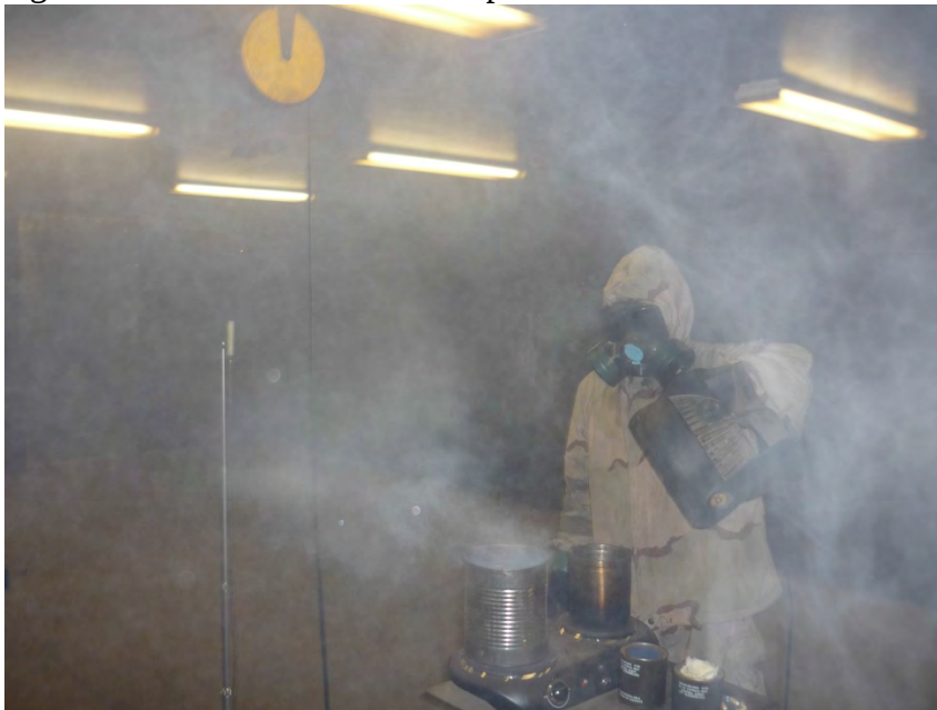
CS being blown by hand held fan.
