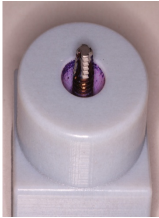
Figure 3. Fabricated resin model of a circumferential bony defect.
