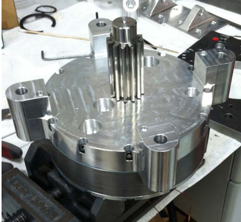
Fig. 19 Fully assembled MREA
