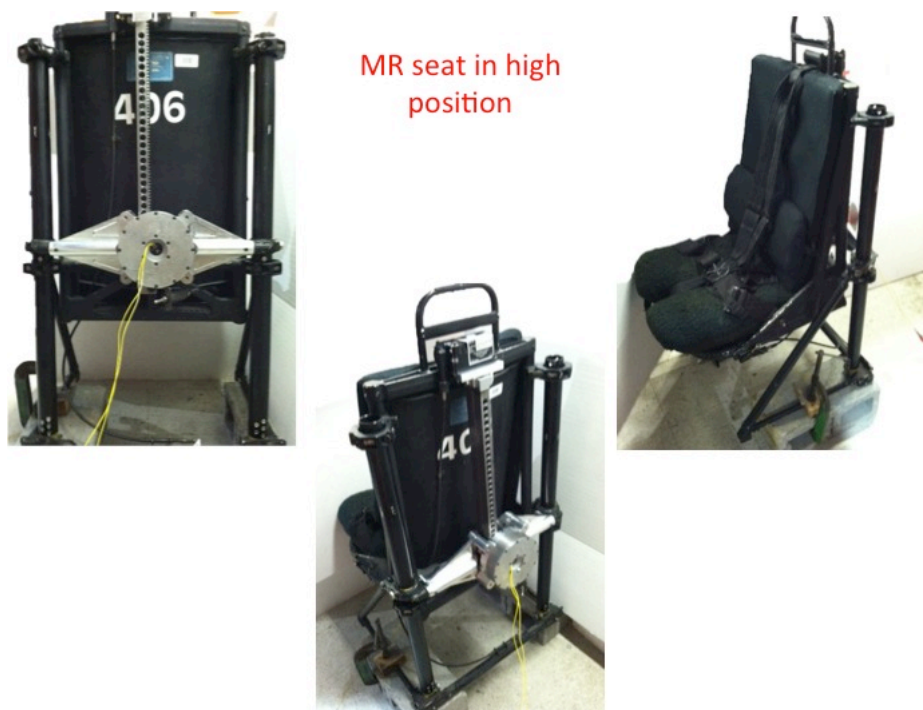
Fig. 58 Iron bird test seat with MREA: high position
