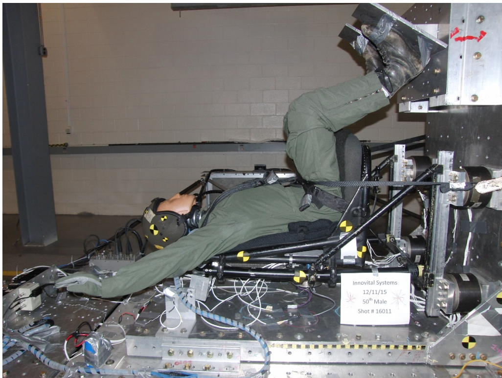
Fig. 86 Posttest photo for test no. 3, 50th percentile male occupant and 42 ft/s crash velocity
