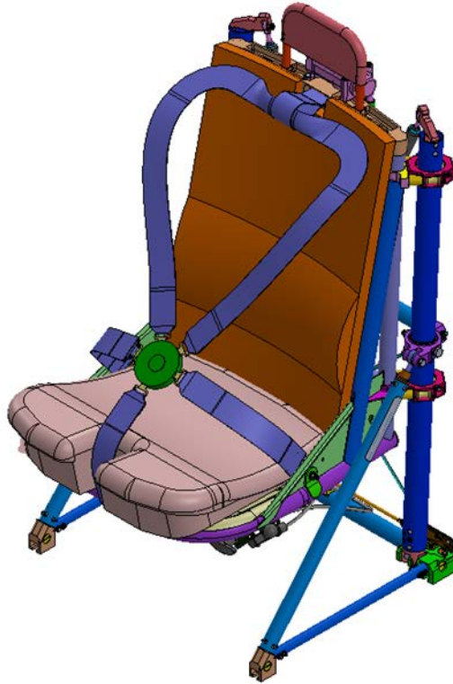
Fig. 48 MH-60R seat manufactured by BAE Protection Systems (formerly Simula, Inc.), front isometric view
