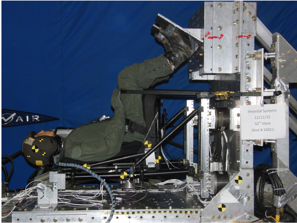
Fig. 85 Pretest photo for test no. 3, 50th percentile male occupant and 42 ft/s crash velocity
