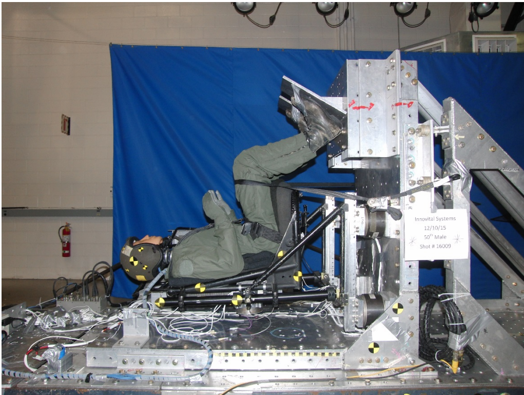
Fig. 78 Posttest photo for test no. 1, 50th percentile male occupant and 21 ft/s crash velocity
