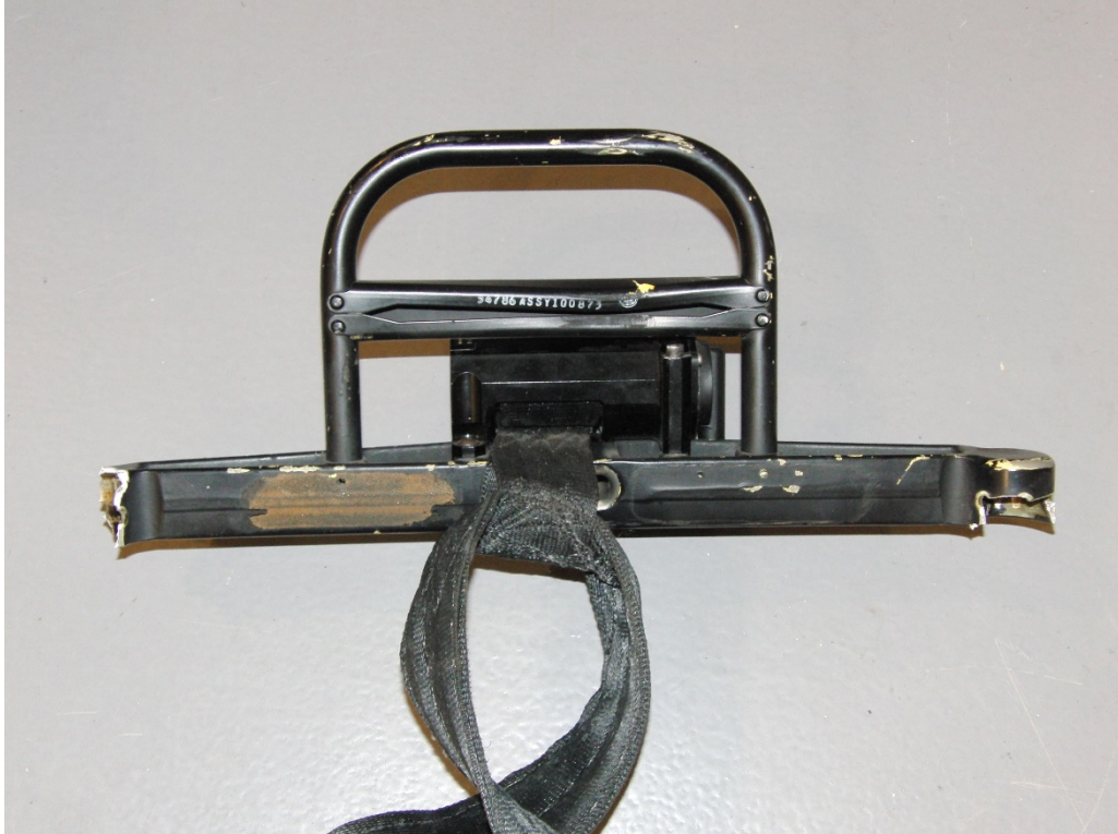
Fig. 88 Posttest photo for test no. 3 showing top crossbar and headrest completely free from seat back
