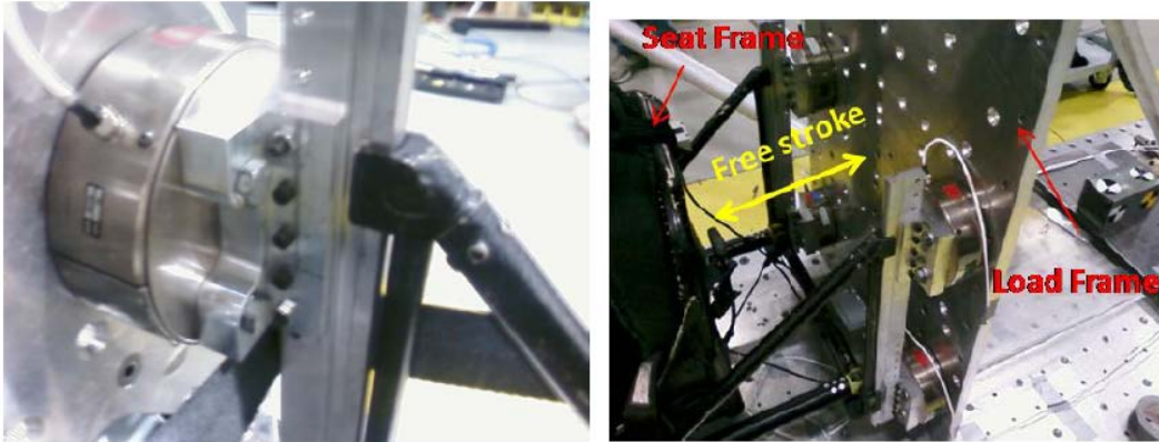
Fig. A-5 Seat attachment to mounting tracks
