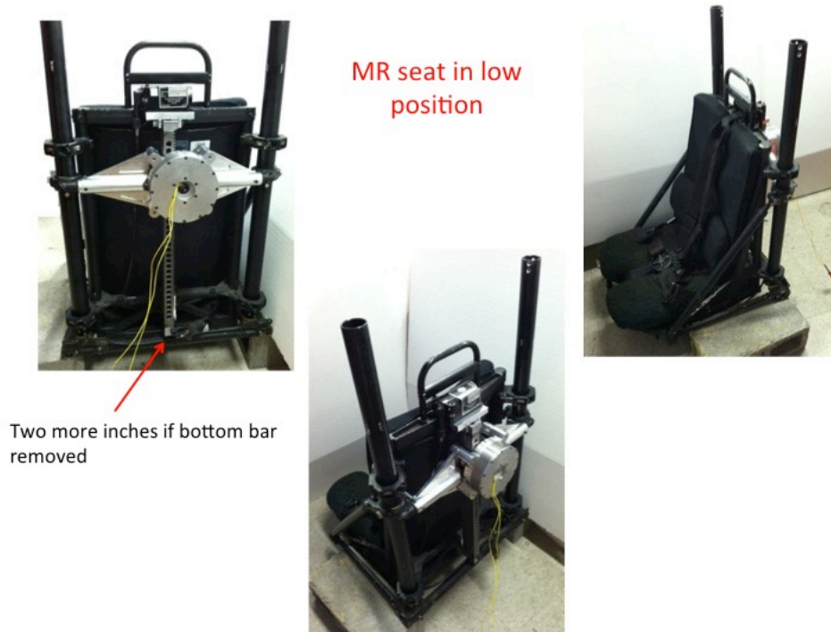
Fig. 57 Iron bird test seat with MREA: lower position
