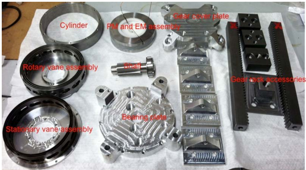
Fig. 18 MREA and motion conversion components
