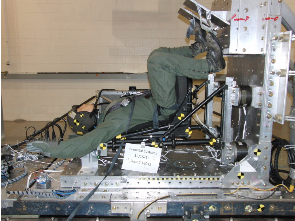
Fig. 90 Posttest photo for test no.4, 50th percentile male occupant and 42 ft/s crash velocity
