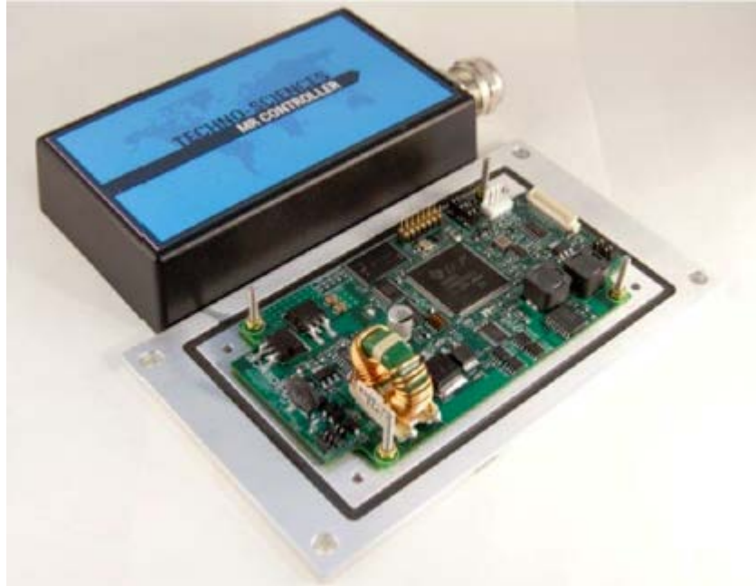
Fig. 75 PCB integrated into mechanical packaging
