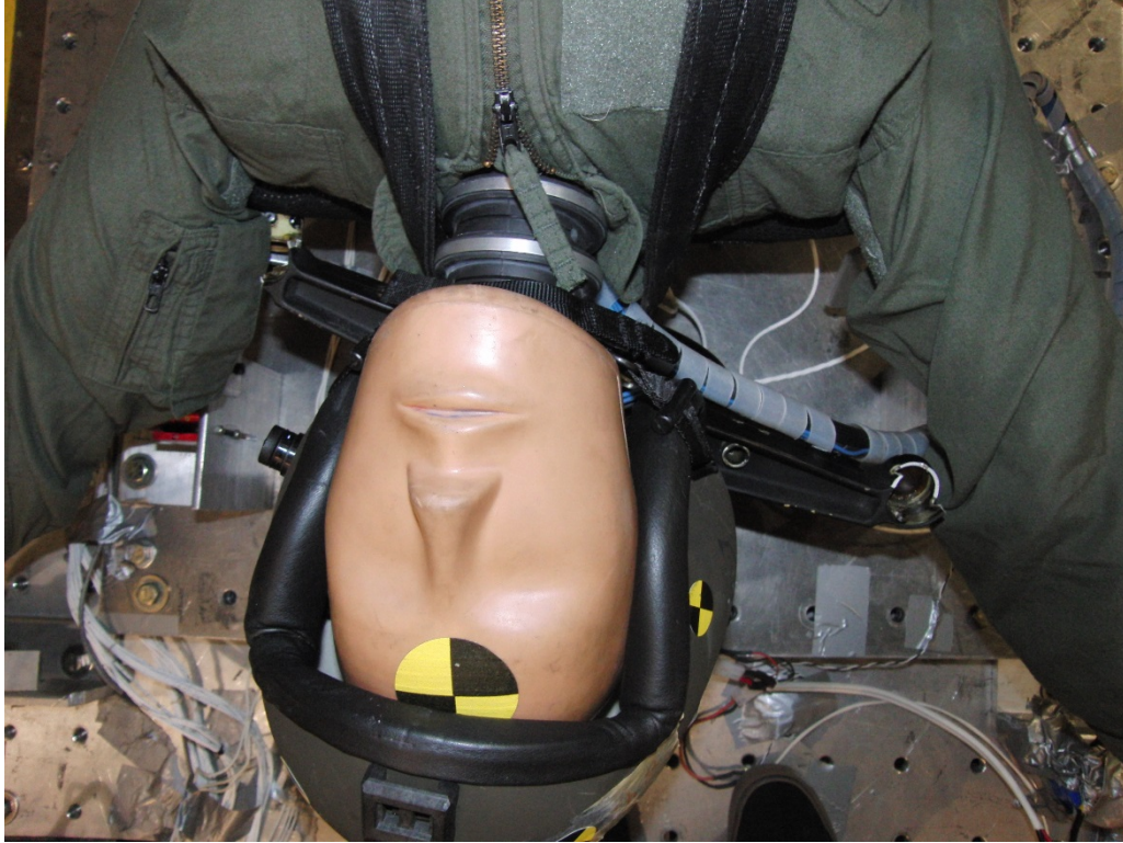
Fig. 87 Posttest photo for test no. 3 showing top crossbar broken off of seat back
