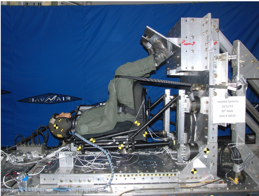
Fig. 81 Pretest photo for test no. 2, 50th percentile male occupant and 34 ft/s crash velocity
