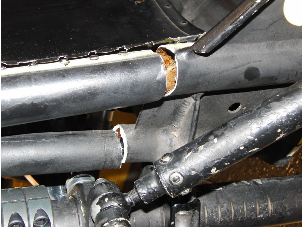
Fig. 92 Posttest photo for test no. 4 showing close-up of broken seat pan
