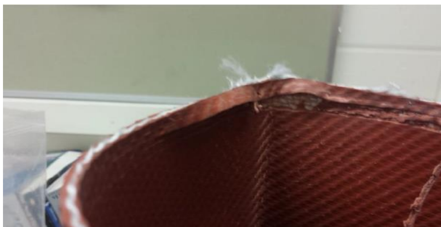
Figure 59: Delaminated Fire Hose Post Test
