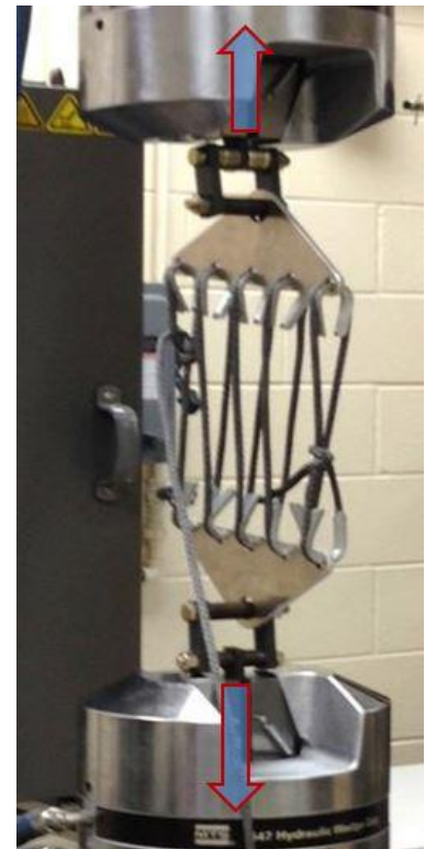
Figure 9: Block and Tackle Tensile Tester Setup
