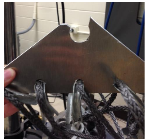
Figure 11: Block and Tackle Tensile Test Failure Location
