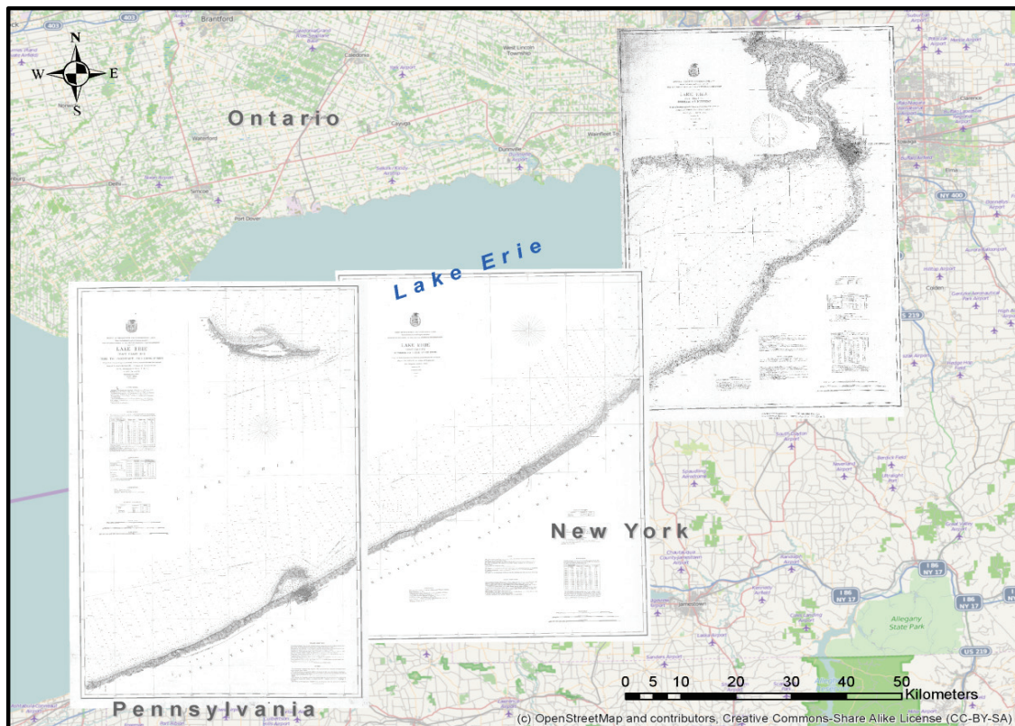
Figure 6. Final transformation of 1870s Lake Survey Charts Numbers 1, 2, and 3 to UTM Zone 17 coordinate system. Background from Esri Maps and Data.
