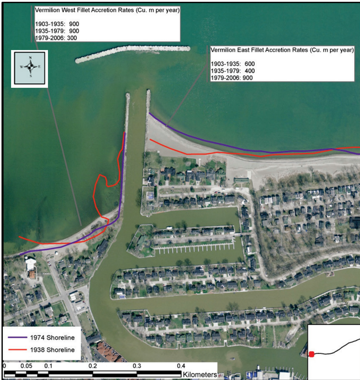
Figure 33. Historic shorelines and accretion rates at Vermilion Harbor, OH (inset map shows position along shoreline between Vermilion and Lorain, OH).
