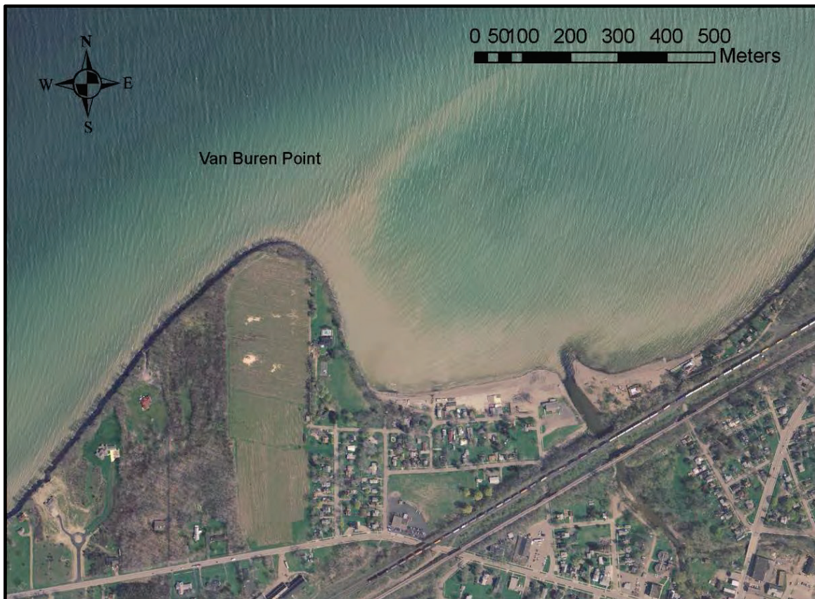
Figure 3. Sediment plume rounding Van Buren Point, NY. The shore along the bay consists of till overlain by lacustrine deposits. Photography: 2004 Chautauqua County 24-inch (in.) Resolution Natural Color Orthoimagery from NYSGIS Clearinghouse.
