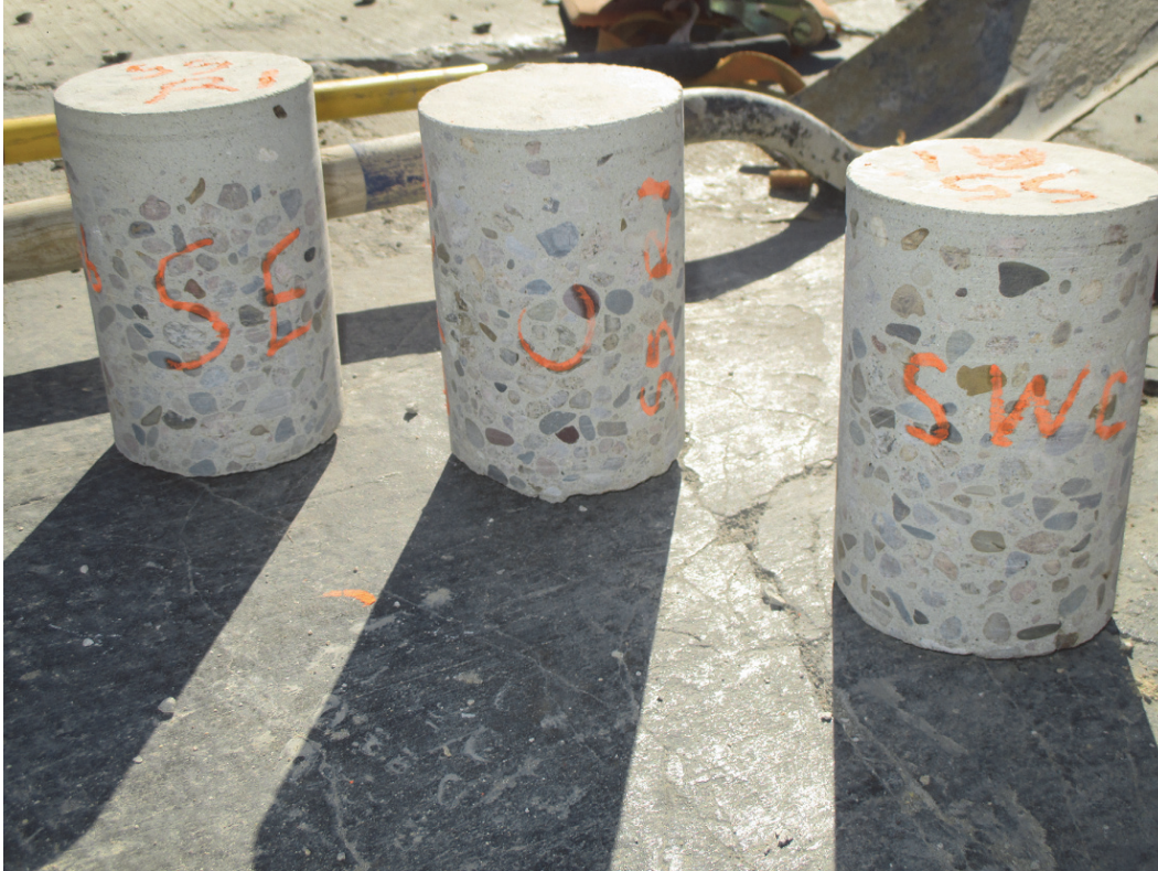
Figure 36. Repair 15 – aggregate segregation of the Rapid Set Concrete Mix® cap.
