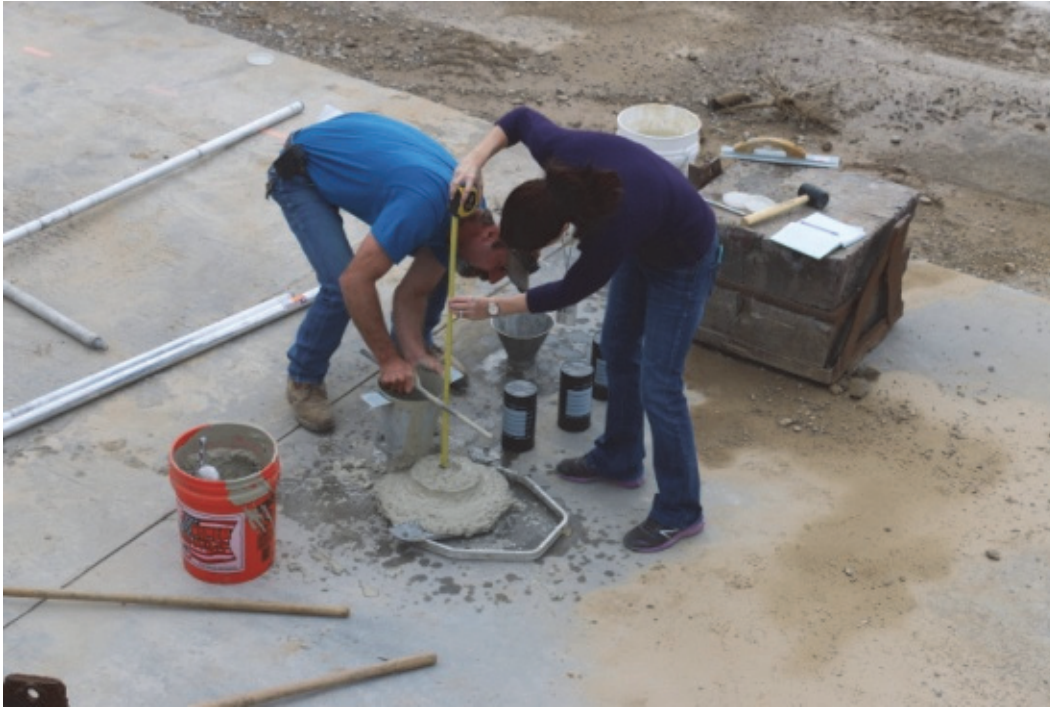
Figure 19. Measurement of slump.
