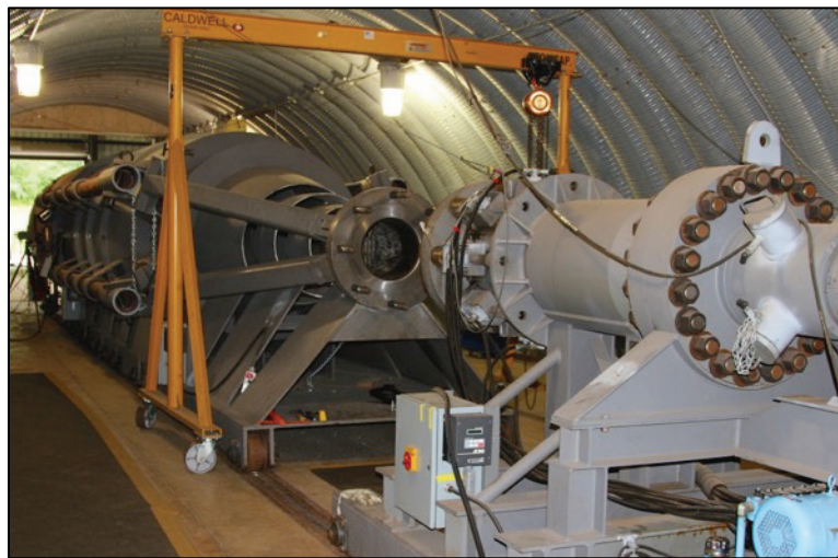
Figure 2.3. Third-scale Blast Load Simulator at the U.S. Army Engineer Research and Development Center (ERDC).
