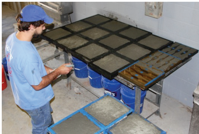
Figure 4.4. Finished HSHDC samples being sprayed with evaporation retardant to prevent moisture loss.
