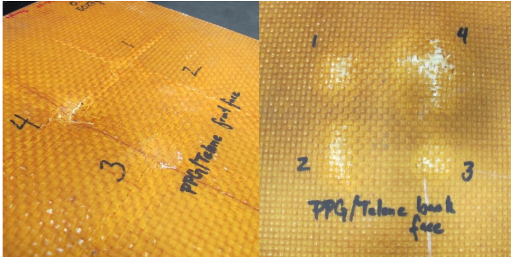
Fig. 20 Front- (left) and back- (right) face damage for the PPG X2-glass-Telene p-DCPD composite
