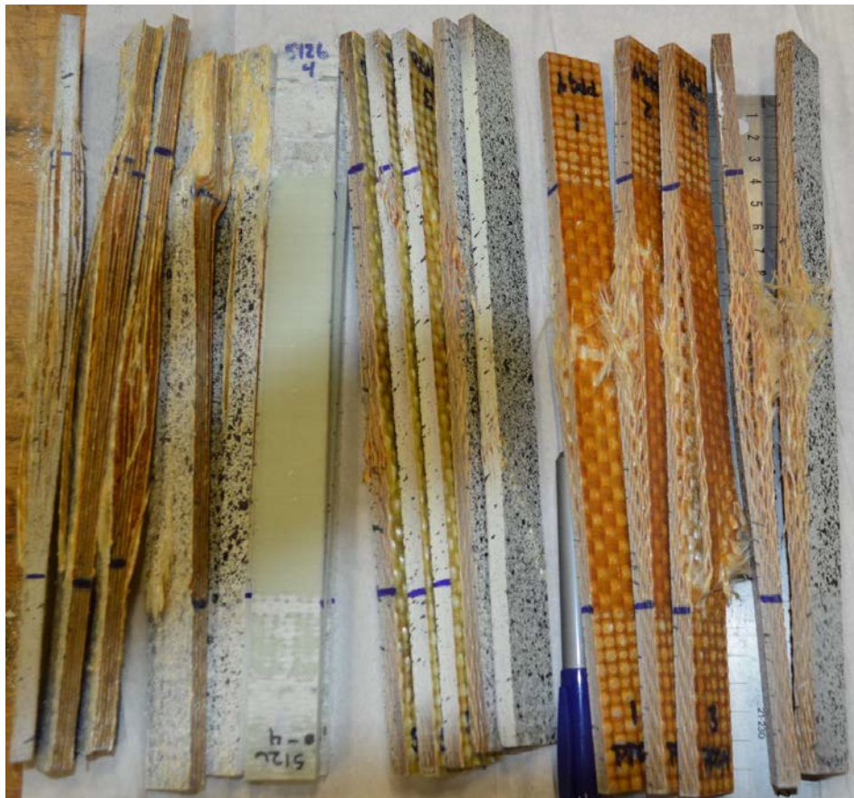
Fig. 7 Group of samples tested in tension: (left) biaxial stitched E-glass-p-DCPD, (center left) biaxial-SC-15, (center right) PPG X2-glass-Spencer p-DCPD, and (right) PPG X2-glass-Telene p-DCPD
